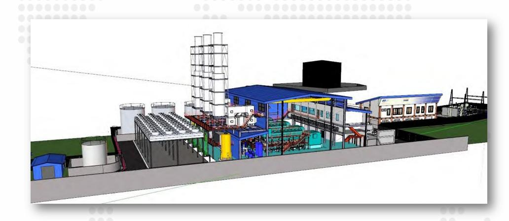
Belawan, N. Sumatra 165MW HFO 4 x MAN 18V48/60TS @ 19.3MW, 500RPM+ 8 x MAN 8L58/64 @ 11MW, 428RPM
